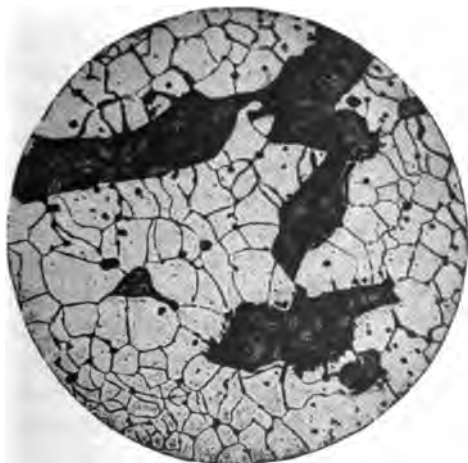
FIG. 196.—Wrought Iron. Transverse Section. Magnification not Stated. (Guillet.)
